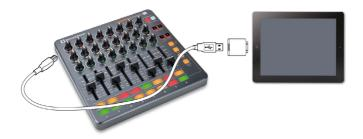
Note: To use the Launch Control XL with an iPad you must switch it to low power mode. To do this hold down both the User and Factory Template buttons and insert the USB cable. Release the Template buttons and press 'Record Arm'.\* Finally press the right arrow button.
